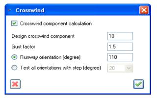
WindRose PRO can be used for calculating crosswinds and to evaluate the correct orientation of a runway. It is also possible to find the best orientation for a new runway. It is possible to specify a designed, or maximum, crosswind component, using the same units of the wind data loaded in WindRose PRO.
